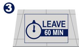
Apply the second coat after 60 minutes of the first coat drying.
