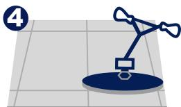
Wipe off excess residue with a cotton cloth or buffing pad after 2 hours. Allow it to cure for 24 hours.
