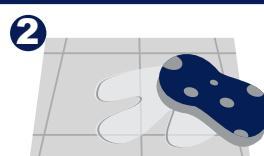
Apply the first coat of Polyglaze PZ Stone Backcoat evenly on the back of the stone using a brush, cotton cloth or sponge.
