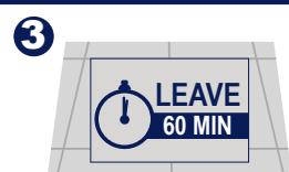
Apply the second coat and allow it to dry for a minimum of 60 minutes before fixing the stone.
