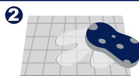
Apply diluted Polyglaze PZ Tile & Stone Cleaner with clean water in 1:1 ratio on the surface using a cotton cloth or sponge.
